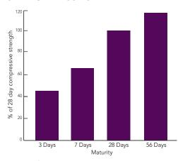
Note: These Concrete Mix compressive strength results were achieved under controlled laboratory conditions, at 23 degrees Centigrade. They should be used only as a guide to potential strength as various factors can impact final strength results.
