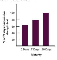
**Note:** This Extra Strength PRO-50 Concrete Mix compressive strength data was achieved under controlled laboratory conditions, at 23 degrees Centigrade. They should be used only as a guide to potential strength as various factors can impact final strength results.
